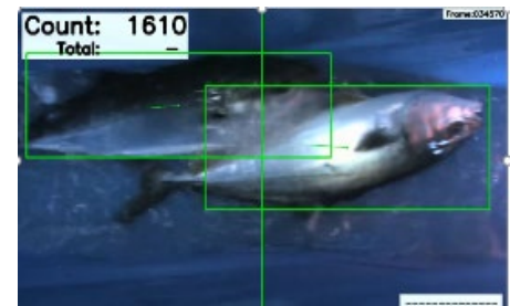
Counting the number of fish using image analysis technology
