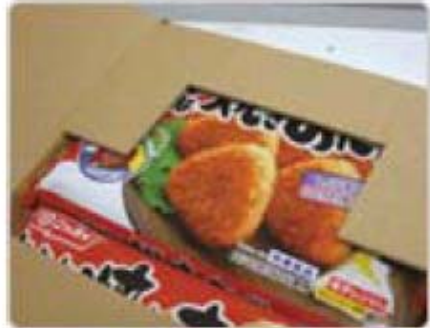
Downweighting by cutting away unnecessary parts of cardboard boxes
